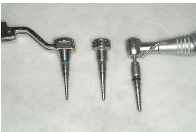
Fig. 2: Different options to drive the expanders are shown in the photo. From left to right: Ratchet wrench, finger wheel and handpiece
